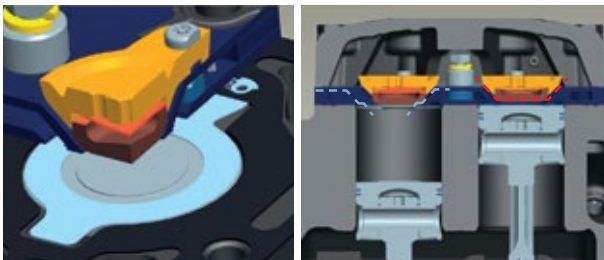
Figure 7: With the Stream design, a larger discharge passage will not increase re-expansion volume leading to the highest efficiency whatever the refrigerant and operating point. A dedicated refrigerant design is not necessary.
