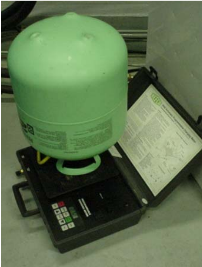
Charging Cylinder on Scale
