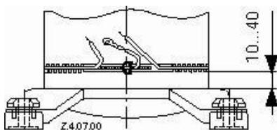
For compressors ZR18K\* to ZR81K\* and ZP24K\* to ZP91K\*, the crankcase heater must be mounted 10 to 40 mm above compressor legs (see **Figure 12**).
