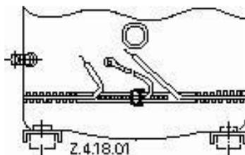
For all other compressor models, the crankcase heater must be mounted below the oil removal valve located on the bottom shell (see **Figure 13**).
