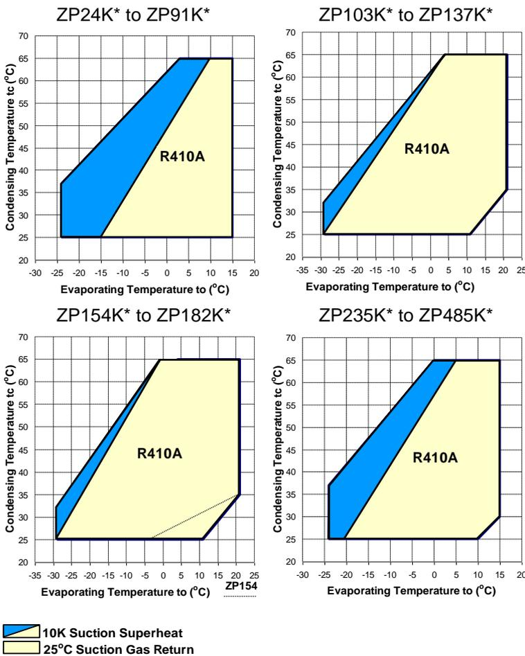
Figure 2: Application envelopes for compressors ZP24K\* to ZP485K\* with R410A
